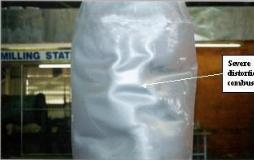
**Severe heat induced distortion evident on combustion duct**
