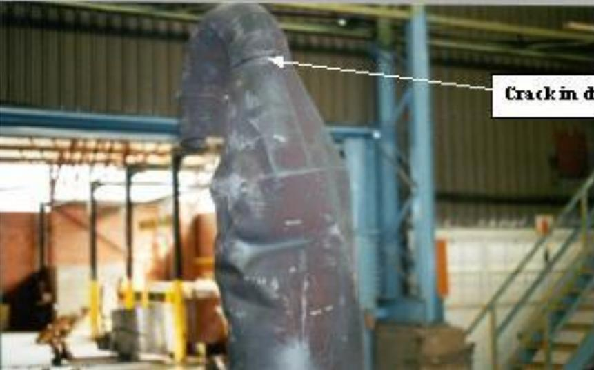
**Crack in duct**
